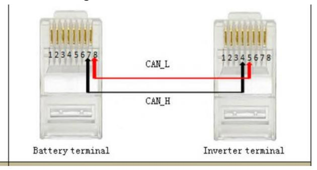
Cat cable needs to be pin7,8 on battery and 4,5 on inverter And connected to the BMS port on the MN AIO.
