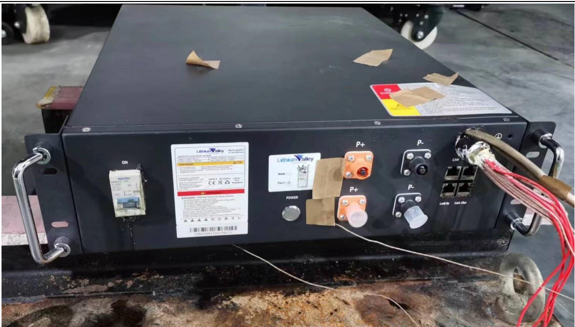
Thermal runaway observed After test
